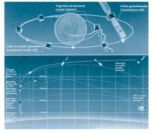
Standard Ariane 5 trajectory for geostationary transfer orbit
