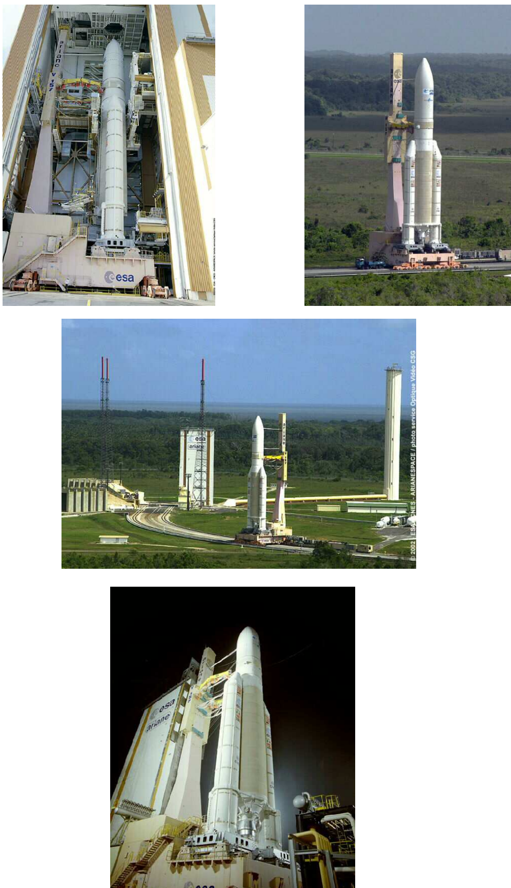
Figure 7.5.5.4.d – Phase 3 operations: transfer to launch pad and chronology
