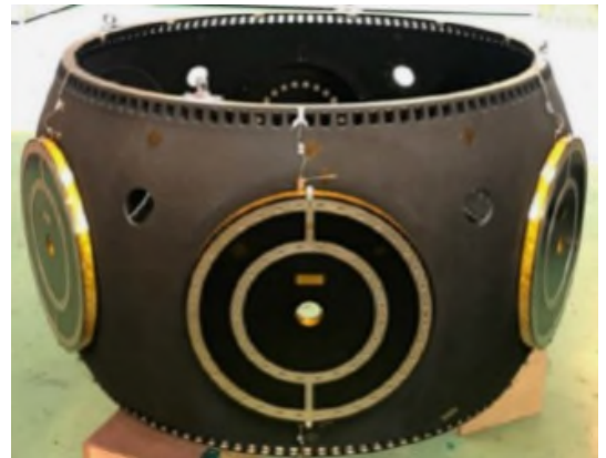
Figure 1.5.2 - Light S/C dispenser illustrative view
