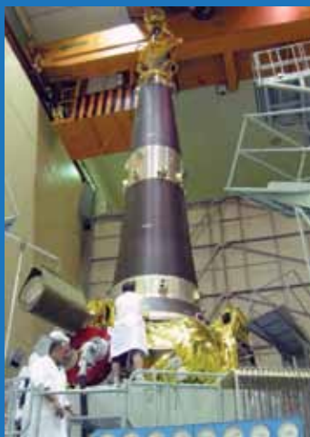
The Soyuz's payload dispenser will carry six Globalstar satellites
