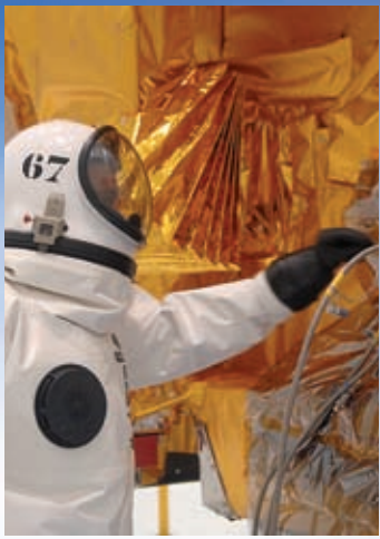
Eutelsat's HOT BIRD™ 9 satellite is fueled at the Spaceport for Ariane 5's next launch
