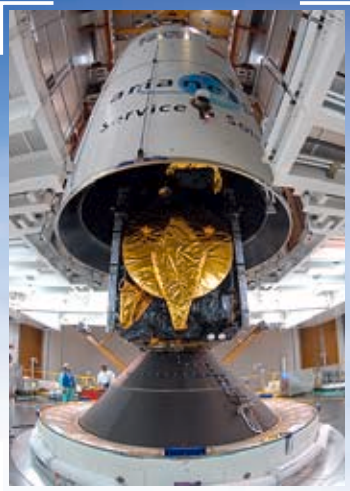
The Skynet 5C and Turksat 3A satellites are integrated on their heavy-lift Ariane 5 ECA
