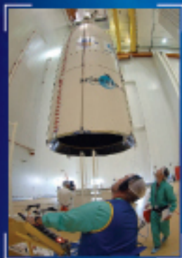
Integration of the SPAIN-SAT and HOT BIRD™ 7A dual payload for Ariane 5
